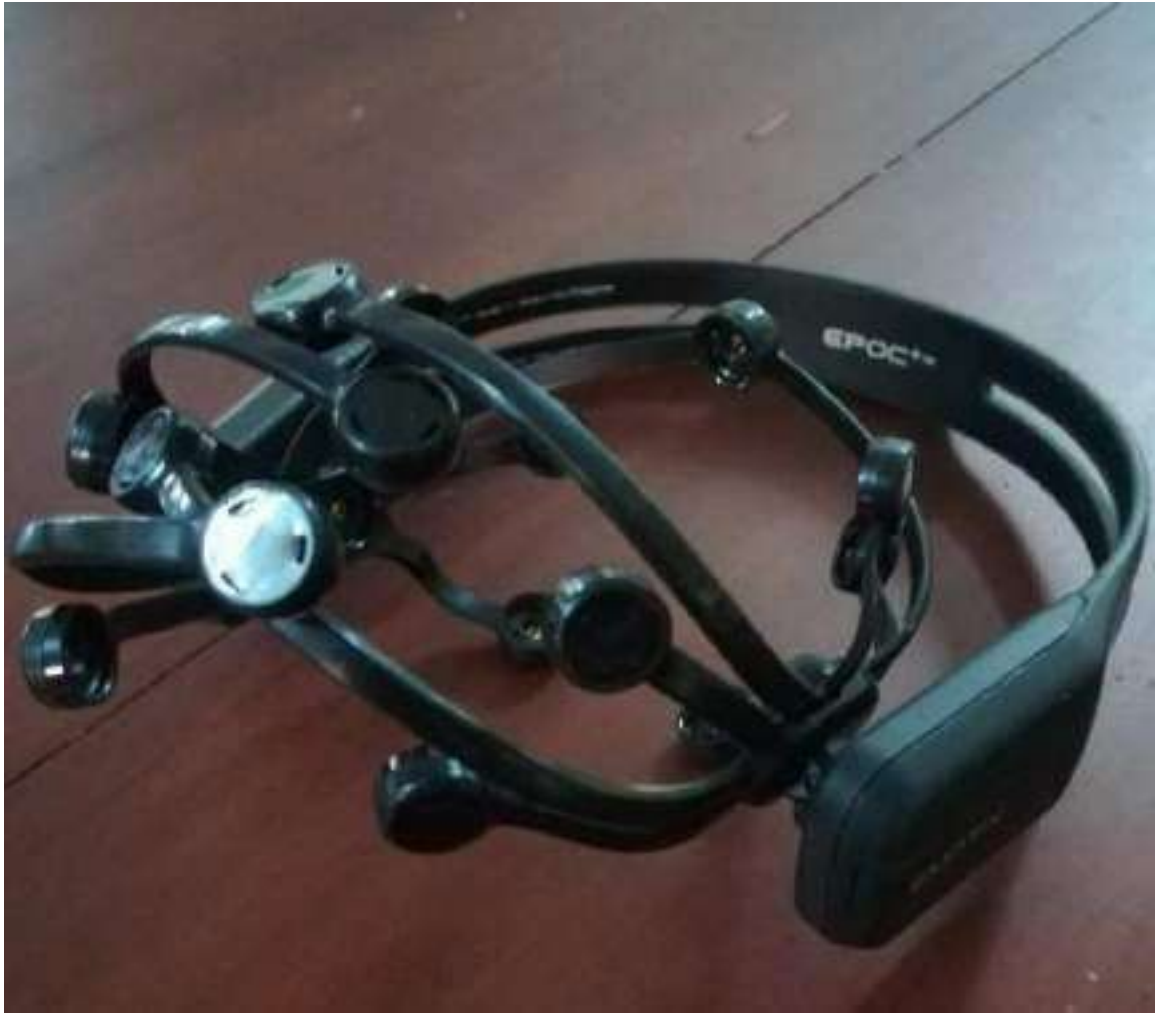
Figure 4. Emotive EPOC mobile EEG headset
