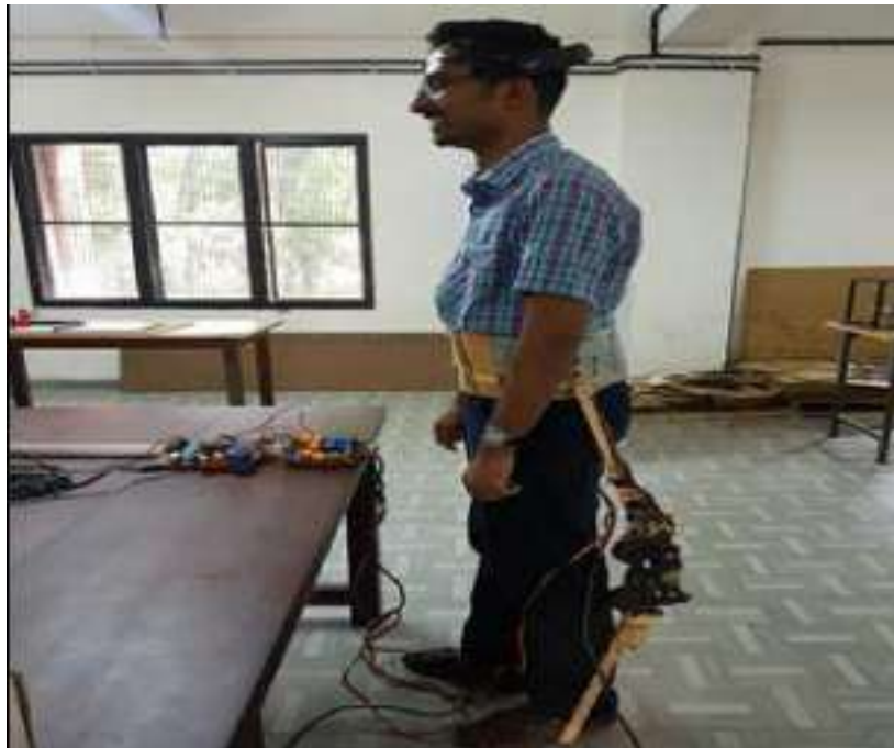
FIGURE 8. Controlling the outer structure of exoskeleton using EEG headset
