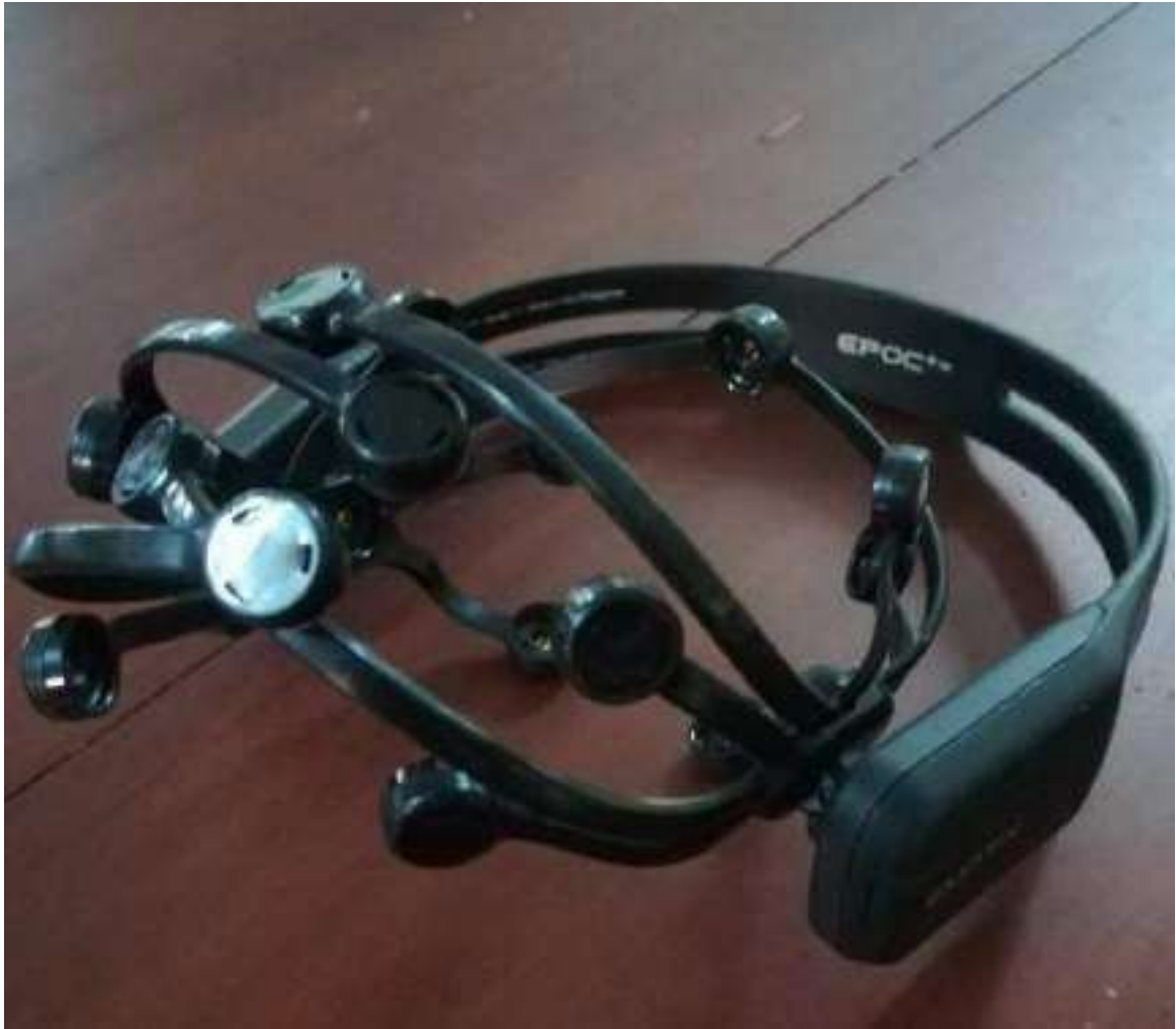
Figure 4. Emotive EPOC mobile EEG headset
