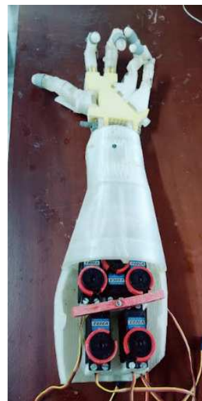
Fig 4 (a) 3D Printed InMoov Robotic Hand (b) Robotic Hand with wearable FABTAC Sensors
