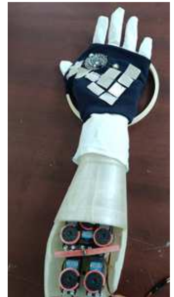
Fig 4 (a) 3D Printed InMoov Robotic Hand (b) Robotic Hand with wearable FABTAC Sensors
