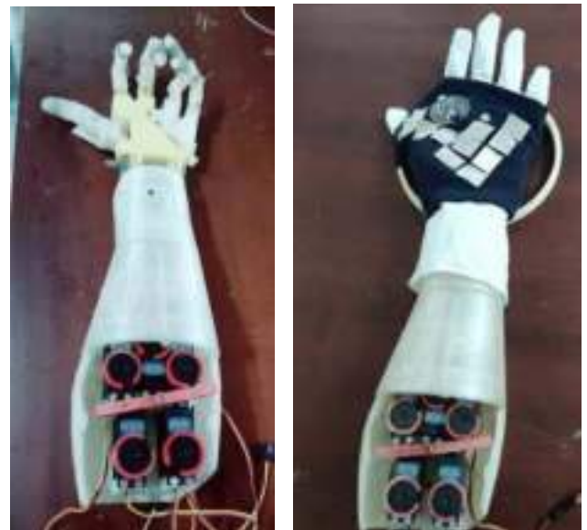
Fig 4 (a) 3D Printed InMoov Robotic Hand (b)Robotic Hand with wearable FABTAC Sensors
