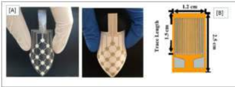
Figure 5.6. (A) Touch sensor based on polyvinylidene fluoride on PED and paper substrates, reprinted from [41] with permission from Elsevier, Copyright (2017). (B) Schematic representation of the RTD sensor, reprinted from [42] with permission from IEEE, Copyright (2019).
