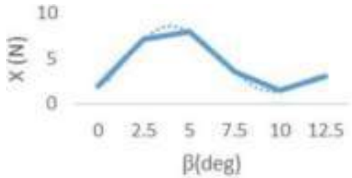
Figure 14. Variation of surge force with angle of attack.
