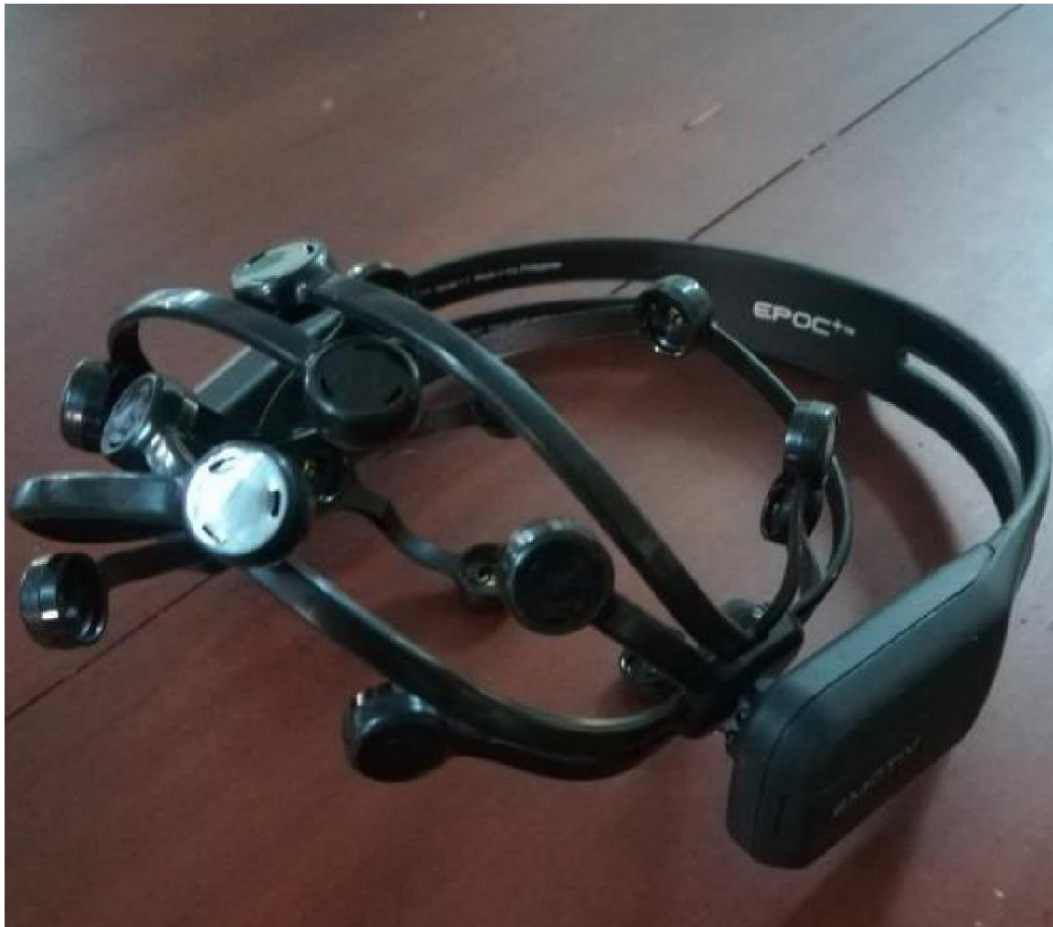
Figure 4. Emotive EPOC mobile EEG headset
