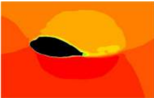
Figure 12. Total pressure contours in pitch.
