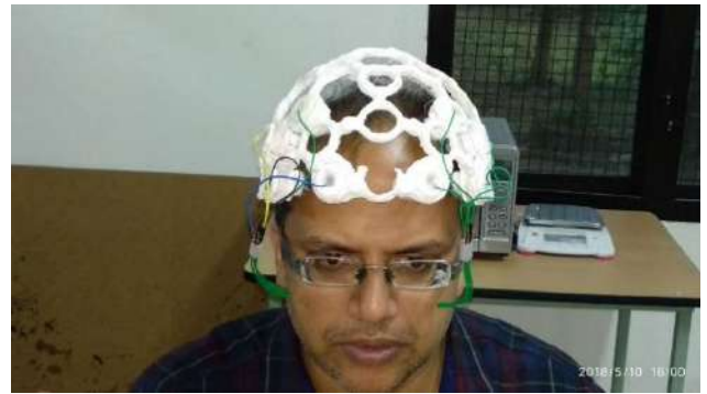
FIGURE 3. Signal acquisition using EEG sensor [21].
