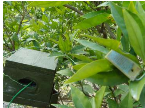
Fig. 2. Deployment of leaf wetness sensor in orange orchard.
