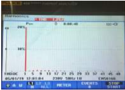
FIGURE 23. Hardware experimental result; THD of output voltage waveform of the ILI.
