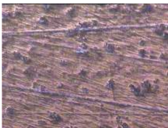
Fig. 16. Microstructure of welded area of EN 24.
