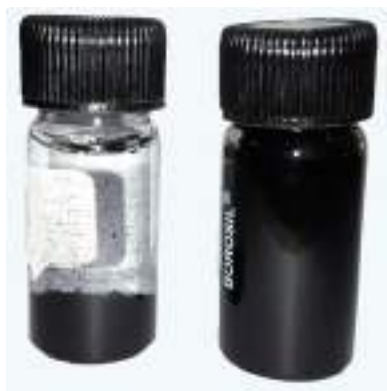
FIGURE 1 Photographs of unmodified and modified multiwalled carbon nanotubes dispersed in water after 7 days [Color figure can be viewed at wileyonlinelibrary.com ]
