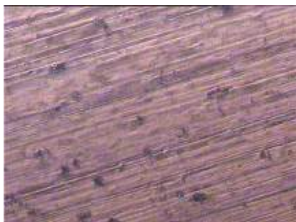
Fig. 15. Microstructure of welded area of EN 9.
