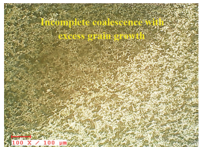
Figure 7. Microstructural analysis of stirred zone of sample 3.
