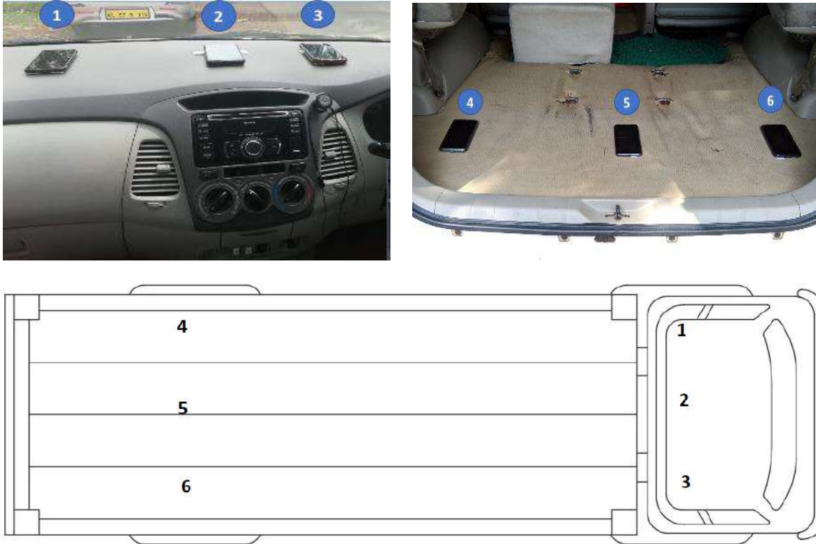
Figure 3: Sensor Positions on SUV and Truck: 1: Front left; 2: Front mid 3: Front right; 4: Rear left; 5: Rear mid; 6: Rear right
