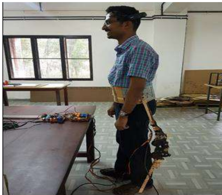
FIGURE 5. Controlling the outer structure of exoskeleton using EEG headset
