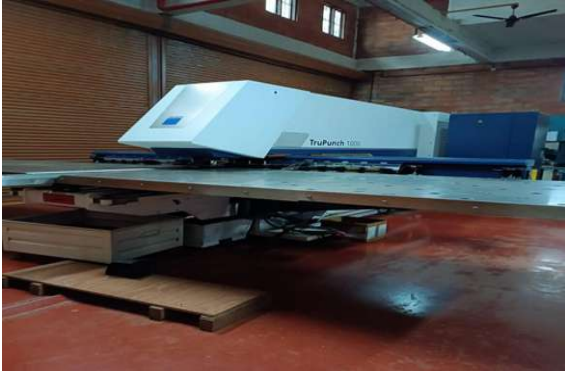
Figure3: Trumpf Punching machine / nibbling machine with CNC
