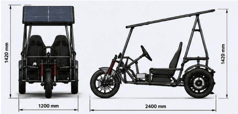
Model of the solar-electric hybrid vehicle (SolarMech Mk.1, SCMS SET). 450W solar array roof, 48V/20Ah LFP battery, 500W BLDC rear hub motor, tubular steel chassis.
